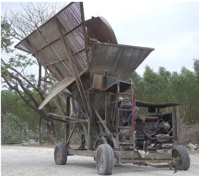
Picture 3.7 Chopping Machine with a Sieve on the Top
