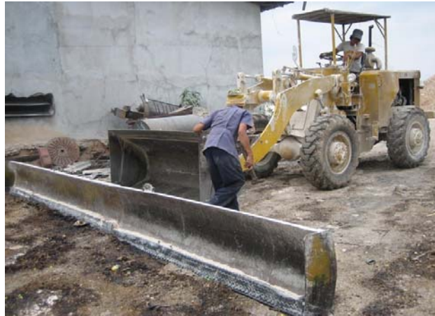
Picture 3.15 Attaching a Dried Chip Collecting Hand to the Bulldozer
